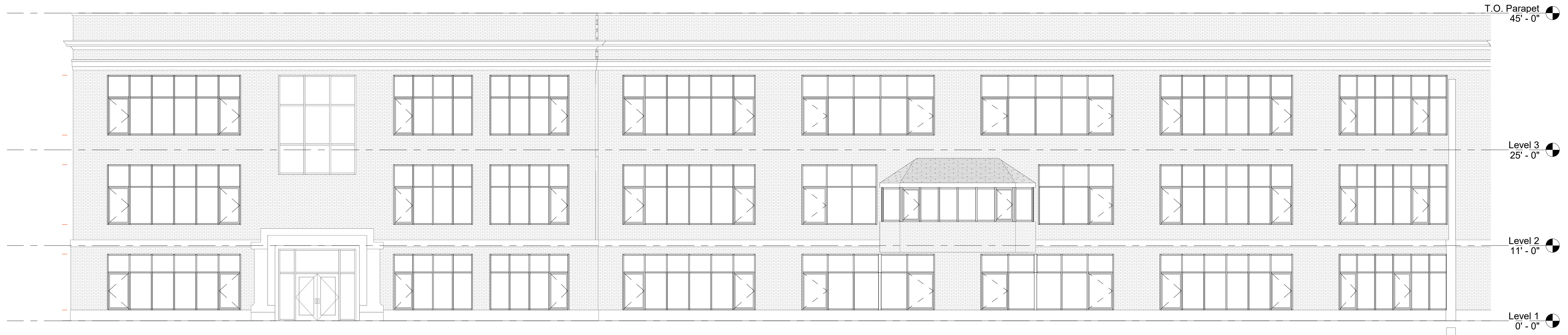
1 Exterior Elevation - East - South Half 1/8" = 1'-0"
