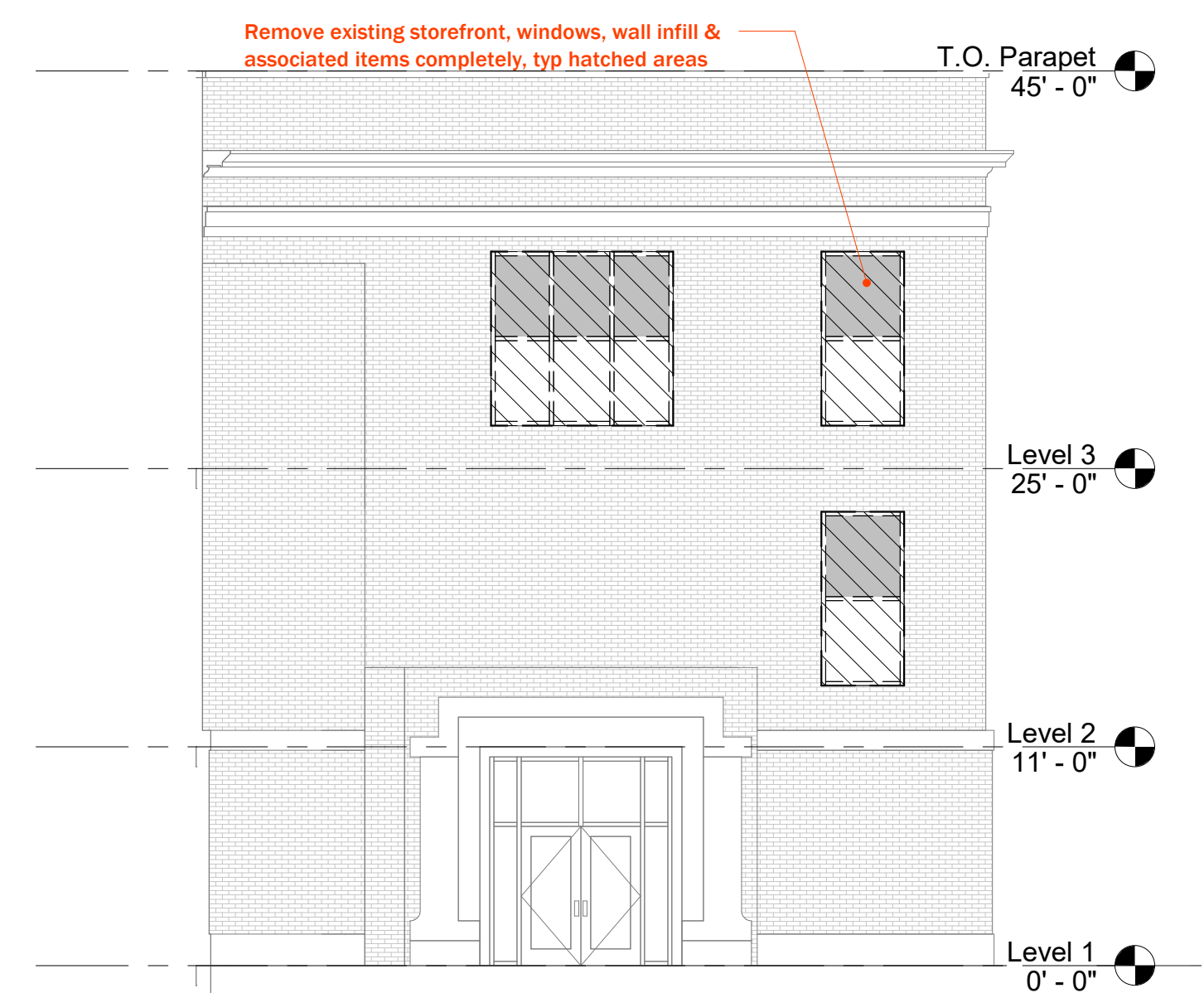
6 Demolition Elevation - NE Corner - South 1/8" = 1'-0"
