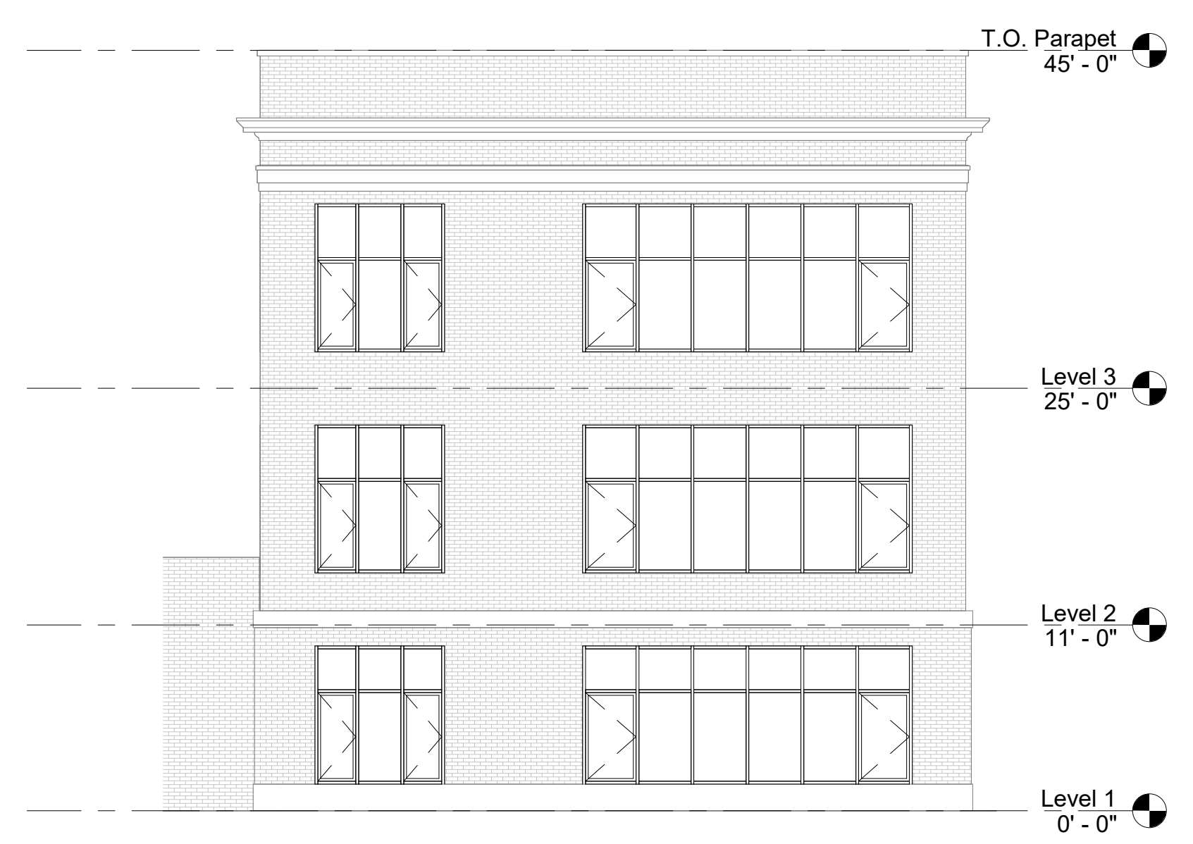
4 Exterior Elevation - East - North Half 1/8" = 1'-0"
