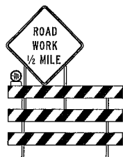
WITH TYPE "A" FLASHING WARNING LIGHT MOUNTED ABOVE TYPE III BARRICADE
