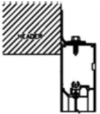
D?:DOOR HEADER SEAL DETAIL no scale
