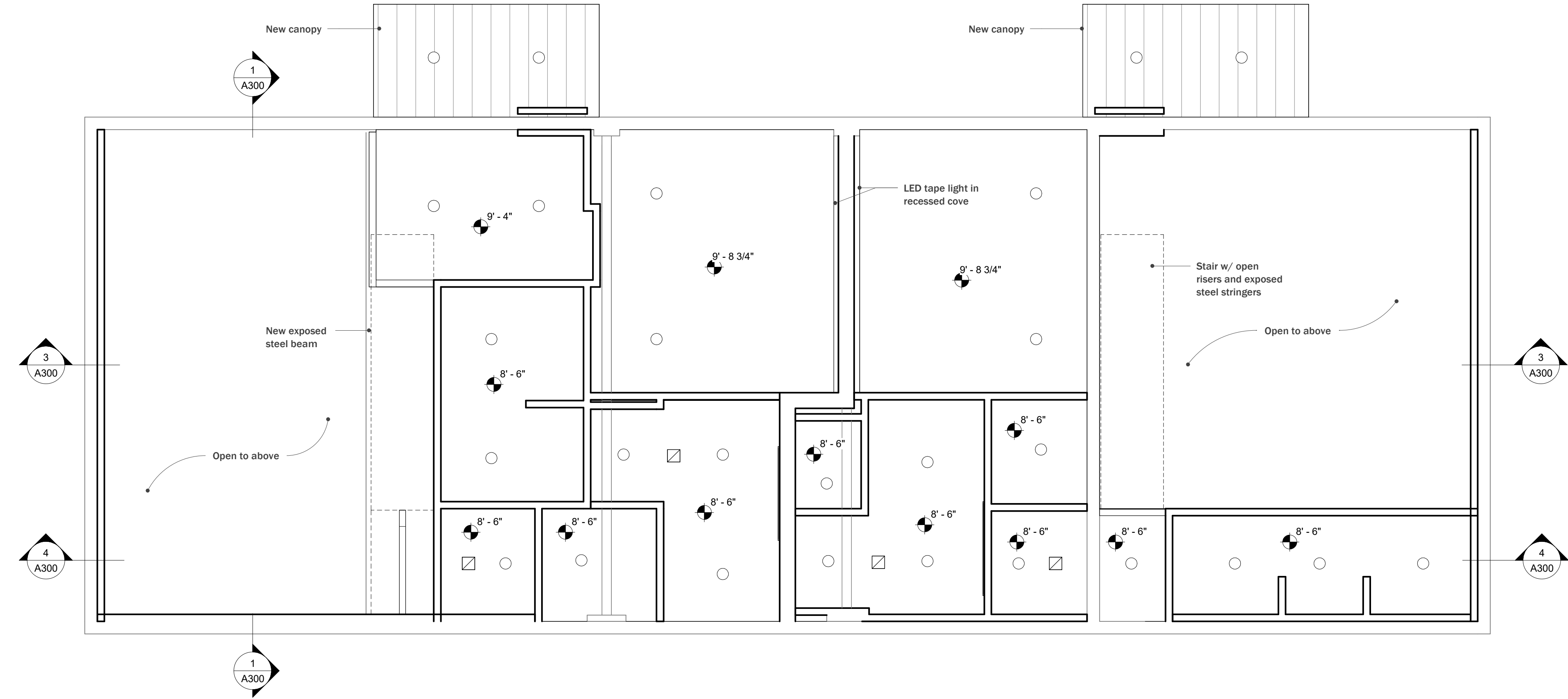
2 Building A Level 1 Reflected Ceiling Plan 1/4" = 1'-0"
