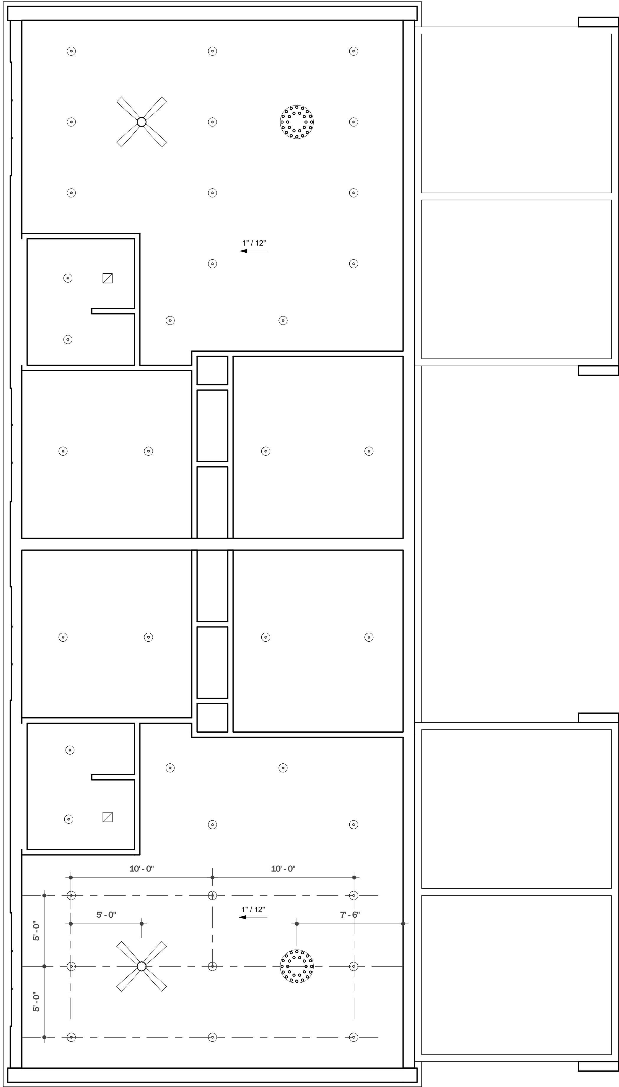
2 Building B Level 2 Reflected Ceiling Plan 1/4" = 1'-0"
