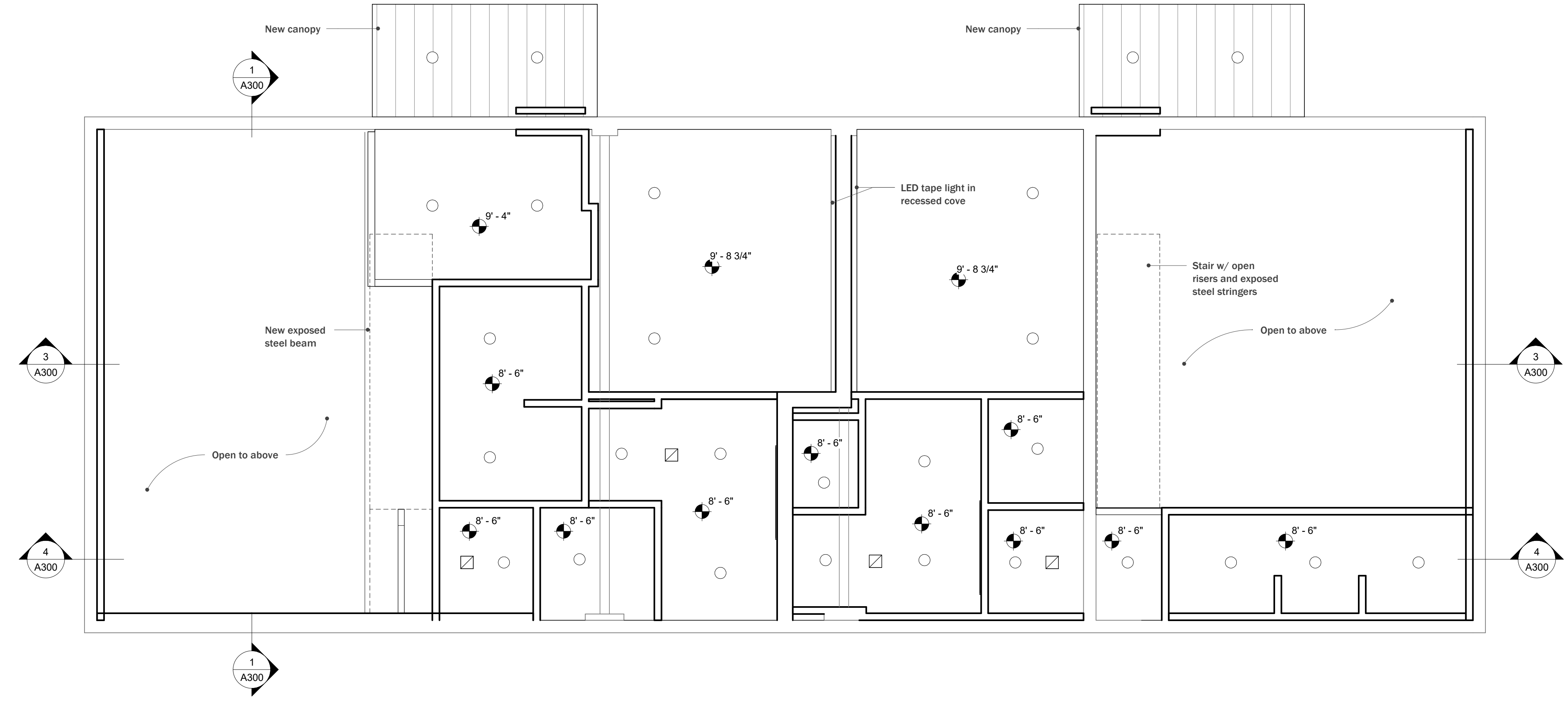
2 Building A Level 1 Reflected Ceiling Plan 1/4" = 1'-0"
