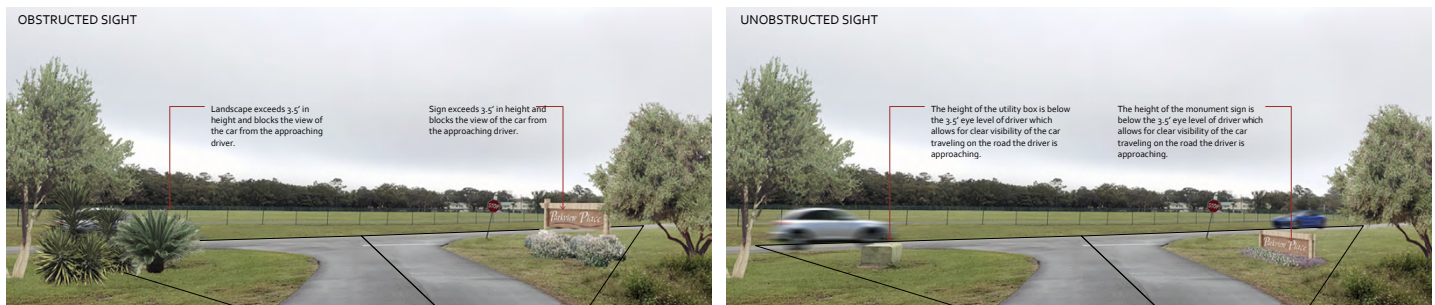
Figure 4: Obstructed and Unobstructed Sight Triangles
